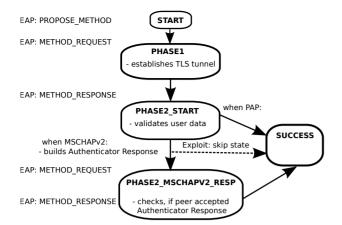
Figure 6: State flow for inner TTLS authentication on the server side. The dashed arrow indicates state skip in EAP-TTLS/MS-CHAPv2 used for the exploit.
