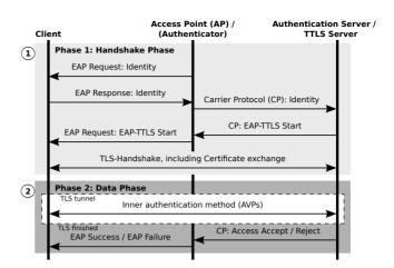
Figure 3: Sample EAP-TTLS Authentication Process
