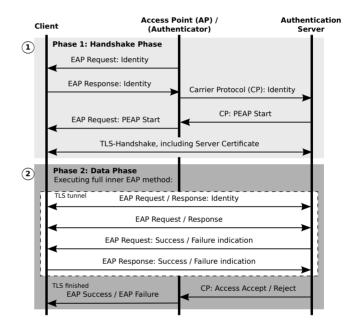
Figure 4: Sample PEAP Authentication Process
