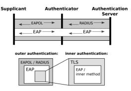
Figure 2: 802.1X Communication and Protocol Encapsulation
